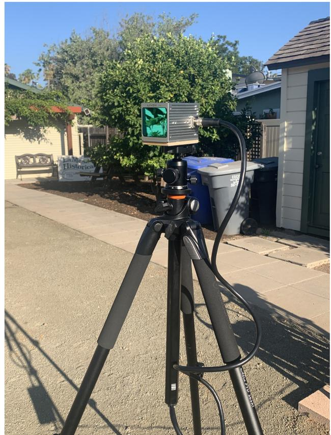
**Figure 1: A Livox Avia LiDAR scanner, adapted for digital heritage scanning using easy to find off-the-shelf components (photo credit: S. Benchekroun).**
